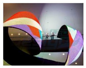
LED displays with 2 way flexibility not only allow the realsation of smoothly produced, uniformly curved shapes like canisters or circles, but can also twist to helical shapes. This opens up many more possibilities for a designer to be creative.
