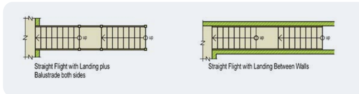
Figure 1.3: Straight stairs with landing.
