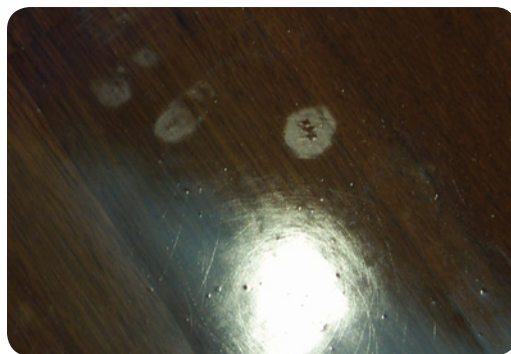
Figure G3: Rejection and contamination in the finish.
