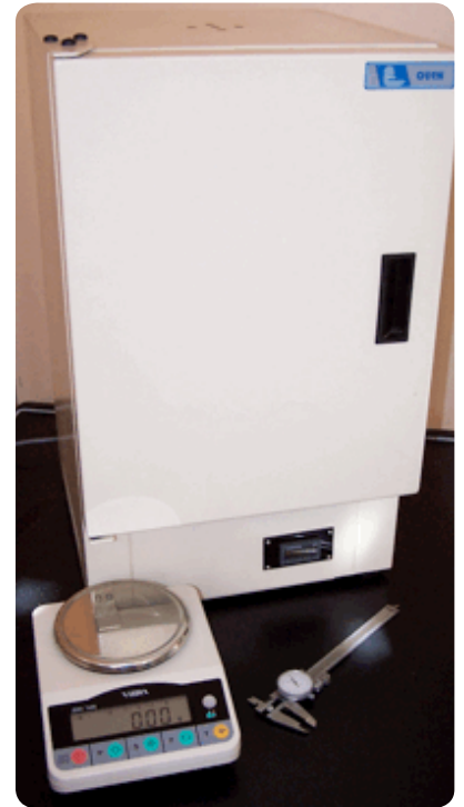
Figure B4: Oven dry testing – Provides the most accurate moisture content test.
