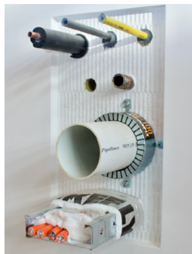
Figure 16: Common products used to seal penetrations in fire-rated lightweight timber-framed walls.
