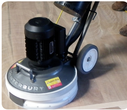
Figure 8.7: Hard plating with the correct attachment.
