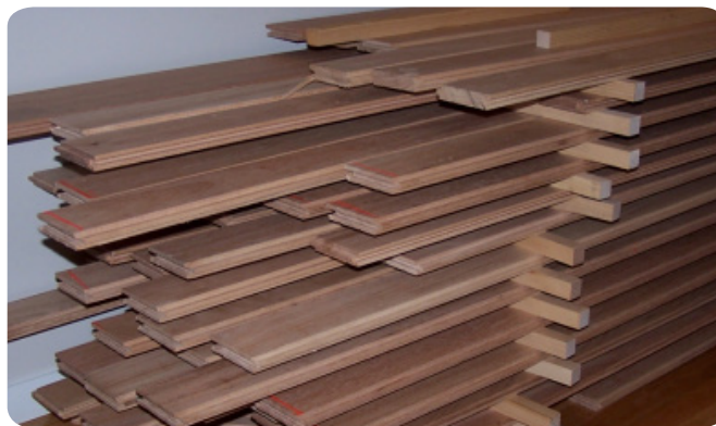
Figure 3.22: Acclimatisation can be effective if product MCs and in-service conditions are known.
