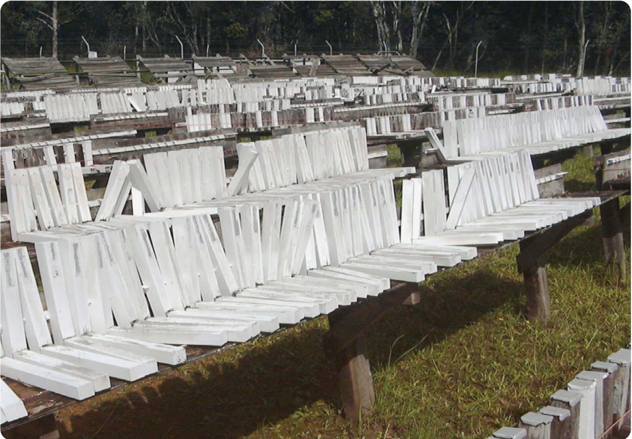
Above-ground durability test site in South-East Queensland.
