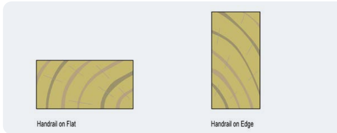
Figure 6.2: Handrails – on flat and on edge.
