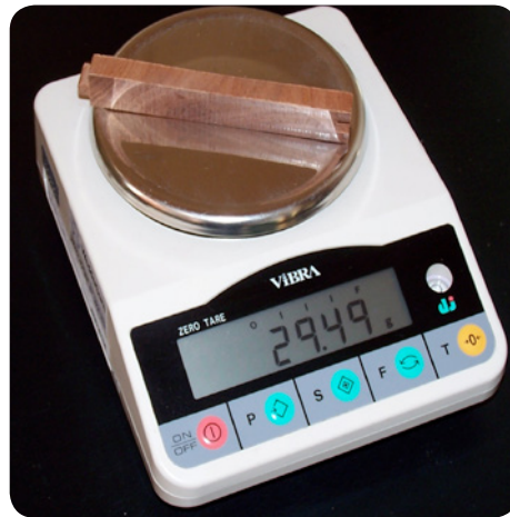
Figure B1: Moisture content measurement.
