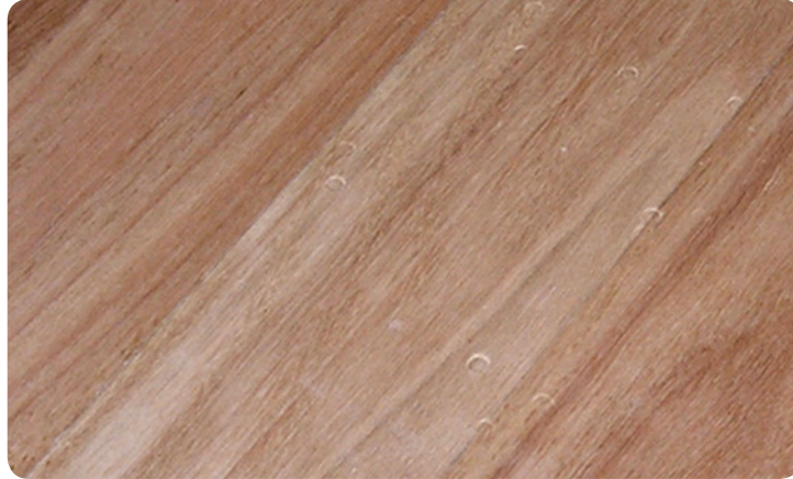
Figure 2.4: Even hard timbers will indent from stiletto heels.
