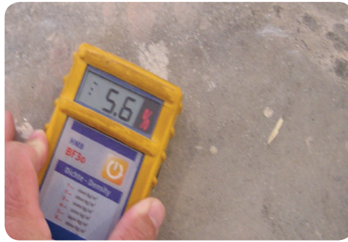
Figure C3: Concrete capacitance moisture meter.
