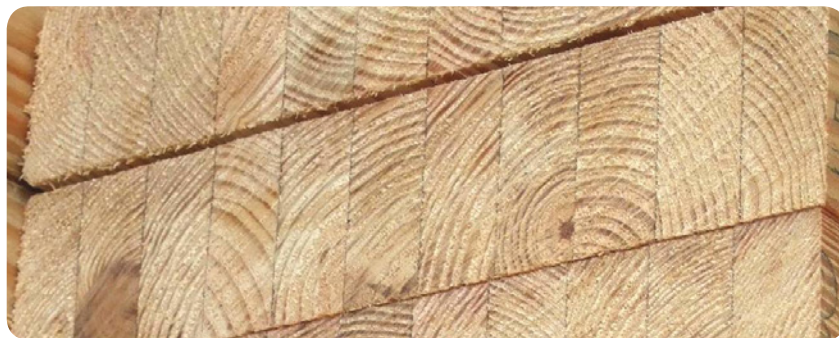
Figure 3: Growth rings in pine glulam.
