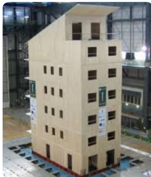
Figure 6.4: 7 storey CLT building on a shake table
