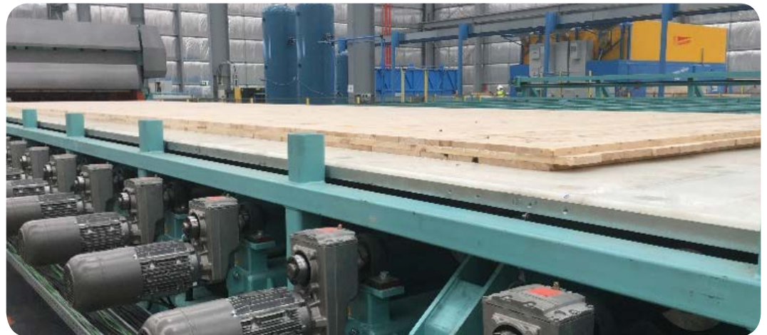
Figure 2.2: XLAM Australia's pneumatic CLT press. Photograph: XLAM
