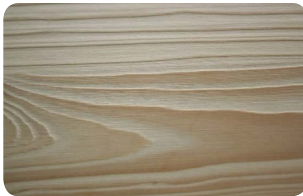
Figure 2.5: Wire-brushed surface of CLT. Photograph: PlanetArk
