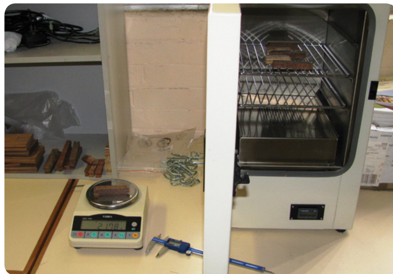
Oven dry moisture content measurement.
