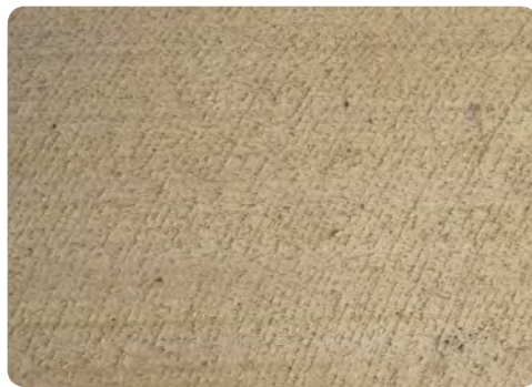
Rough sawn (circular saw).
