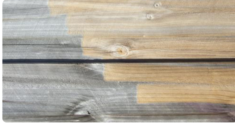
Figure 9: Weathered, grey surface adjacent to unweathered surface.
