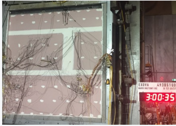
Non-fire side after 180 minutes with full test load applied
