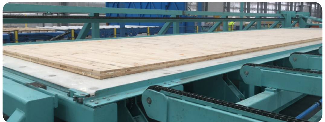
Figure 1.2: 3 layer CLT panel after pressing. Photograph: XLAM Australia
