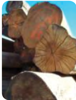
Drying splits in a log.
