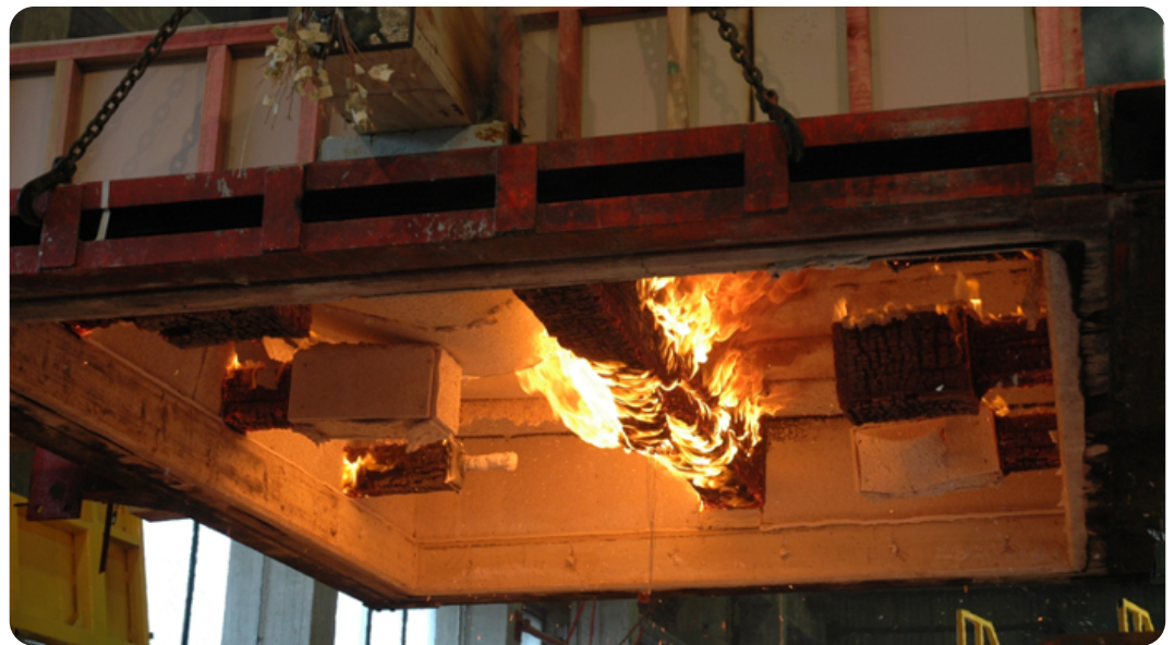
Figure 4.2: Fire resistance test of a post-tensioned timber beam. 5
