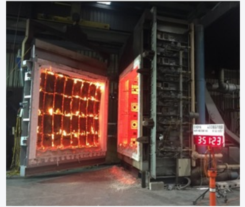
Fire Exposed face 4 minutes after removal from furnace (Test was continued to 227 minutes under reduced load)
