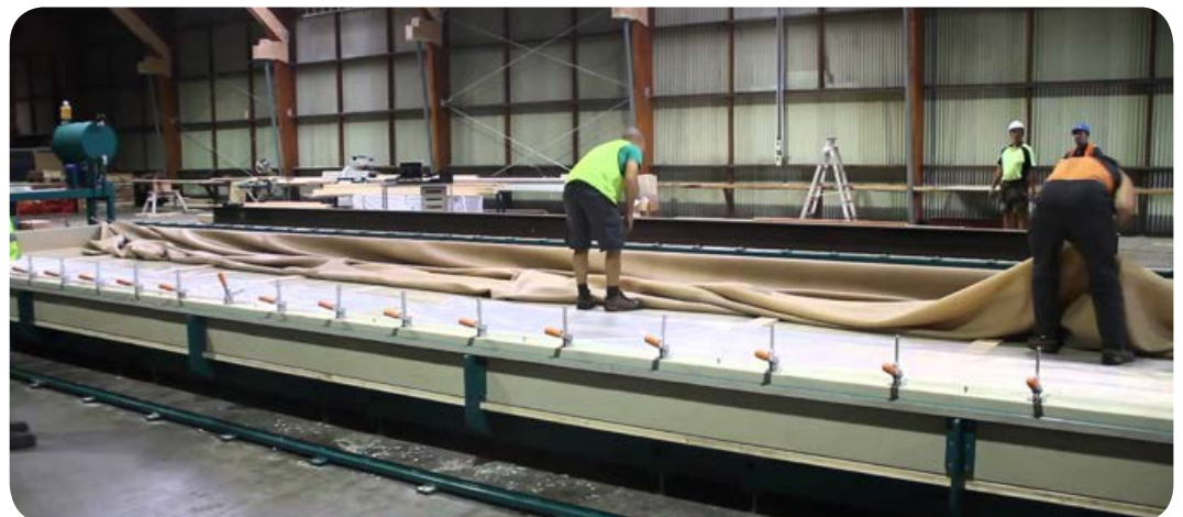
Figure 2.3: XLAM New Zealand's Vacuum Press. Photograph: XLAM
