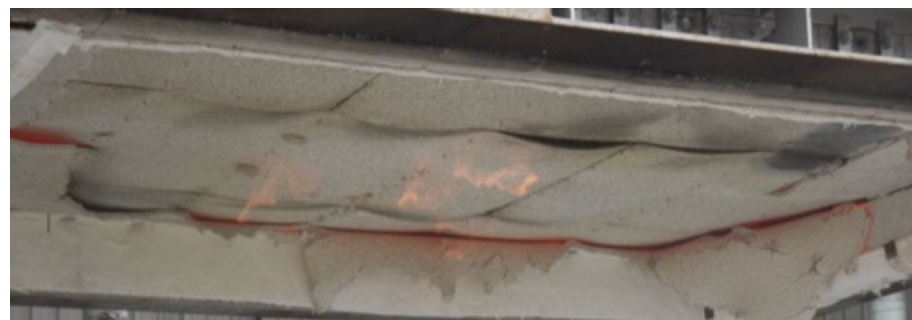
Fire-exposed face after removal from the furnace
