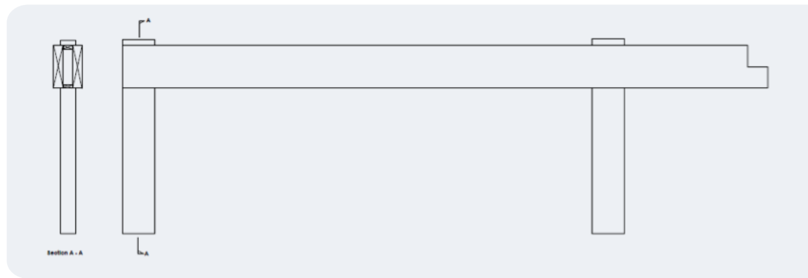
Figure 11: Column and primary beam in one lifting unit.
