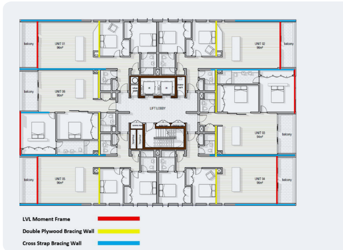
Figure 20: Level 1 Shear Wall Layout
