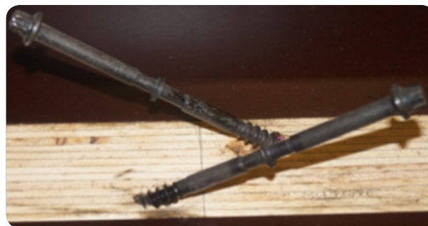
Figure 5.2: SFS screws installed at an angle of \pm 30^\circ (left) and \pm 45^\circ (right).
