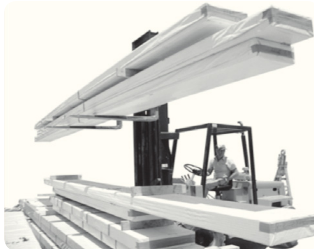
Figure 3.1: Loading and unloading timber beams using a forklift.
