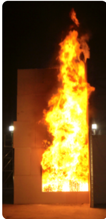
Figure A13: Maximum flame extension estimated to be more than 7 m above opening.
