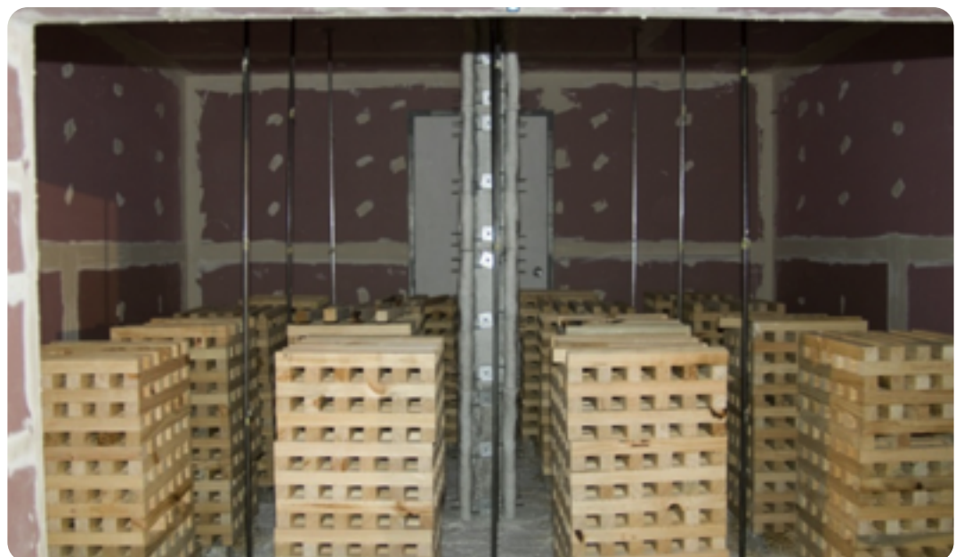
Figure A5: Test enclosure configuration showing protected steel column, timber cribs and thermocouple trees.
