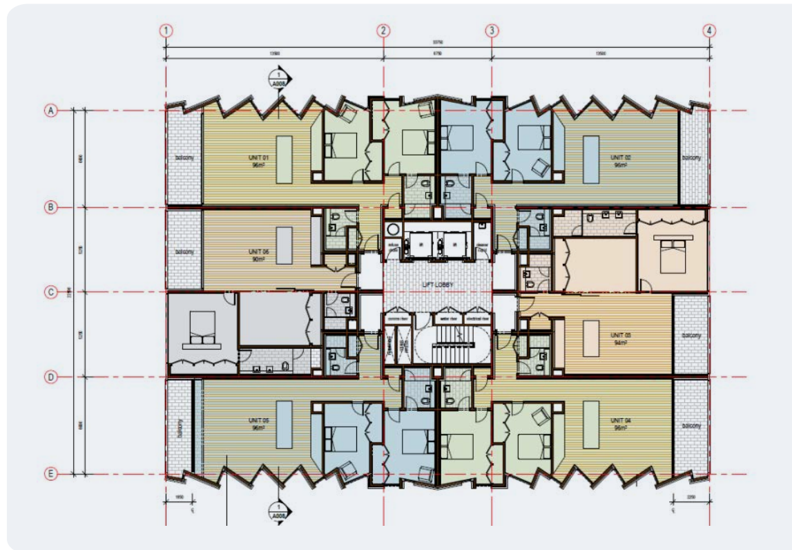
Figure 6.3: Typical CLT apartment layout.
