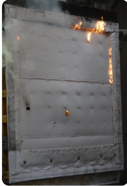
Figure G1: Exposed face of timber-framed plasterboard specimen about three mins after completion of a 90-minute fire resistance test in a free air environment.
