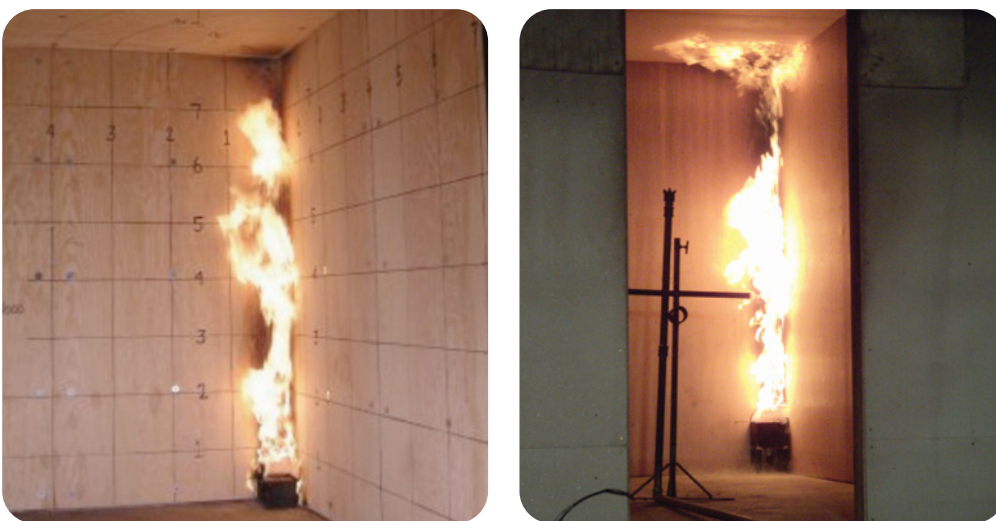
Figure 3: AS ISO 9705 fire tests.
