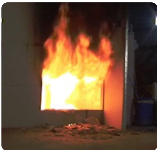
Figure 6: ISO 13785.2 test configuration.
