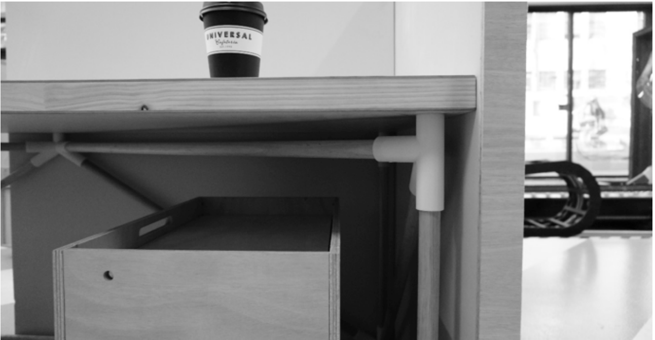
Figure 14: 3D printable joiners and dowels, UTS June 2016.
