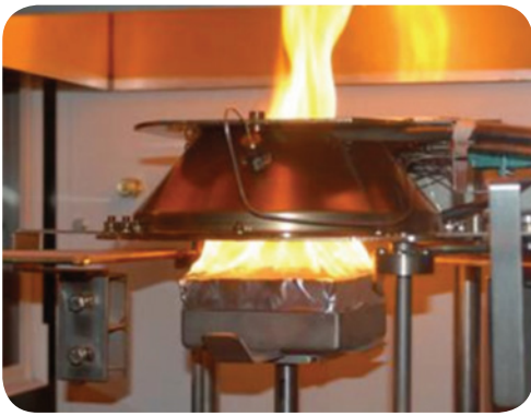
Figure 4: AS/NZS 3837 Cone Calorimeter test.
