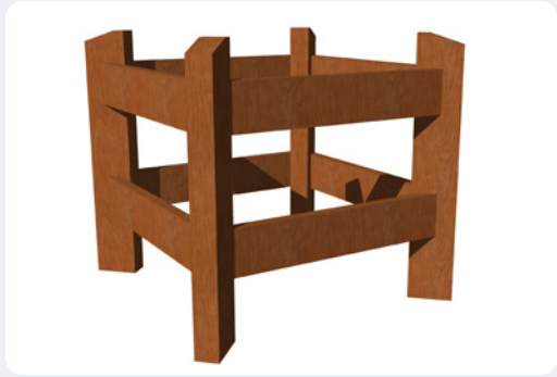
D: Enclosure – Bollards can be in groups and linked with rails to provide protection to trees or structures.
