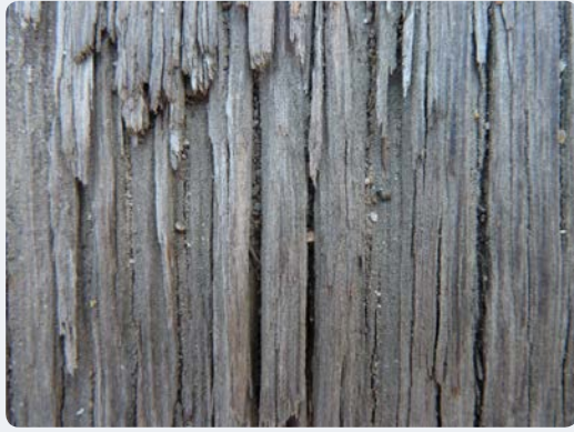
Figure 3.6: Magnified view of a severely weathered hardwood board.
