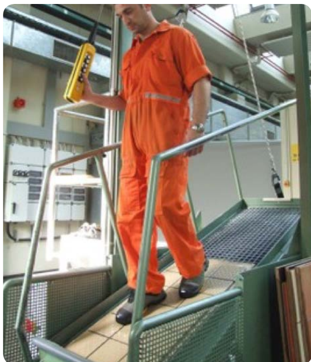
Figure 7.2: Inclining platform From https://oshwiki.eu/wiki/File:ERO-10-06-b-7b.fig1.jpg#file
