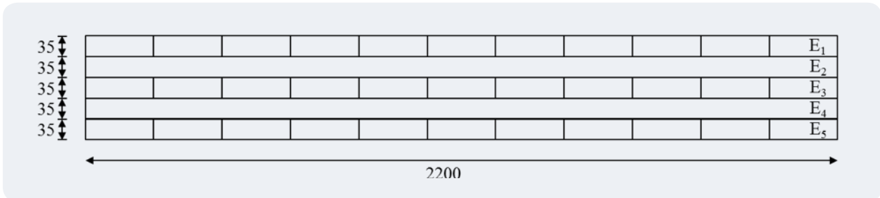
Figure B-1: Cross section geometry of 5 layered CLT panel.
