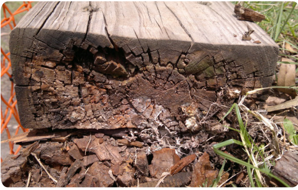
Figure 2.6: Non-compliant CCA treated pine sleepers that failed after 5 years. Sleepers contained excessive amounts of untreated heartwood.
