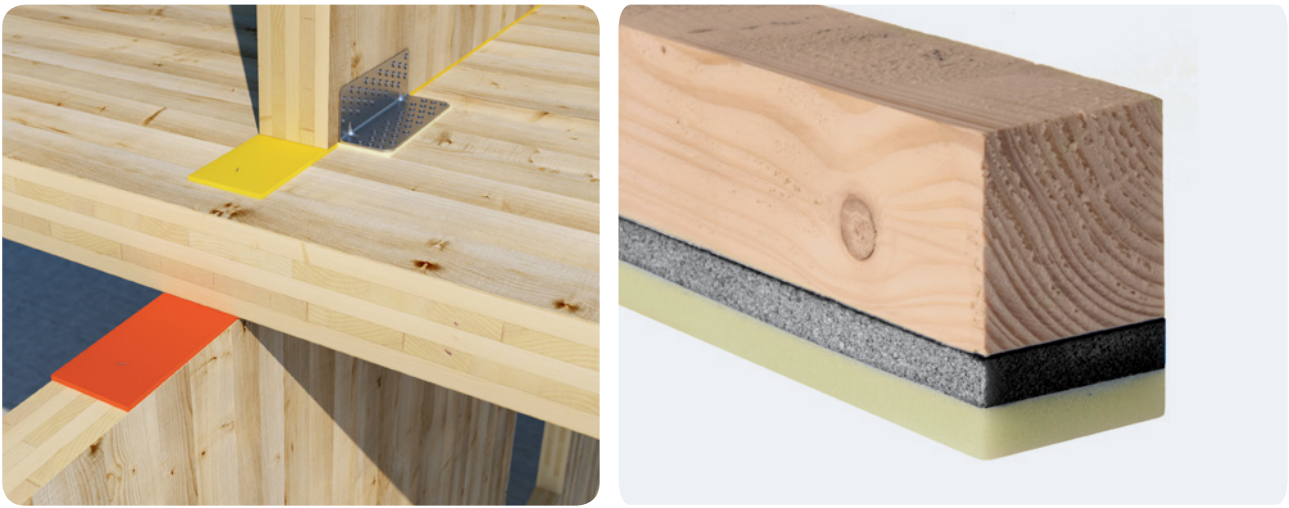
Figure 3.2: Example of acoustic strip in loadbearing connections and of resilient flooring batten
