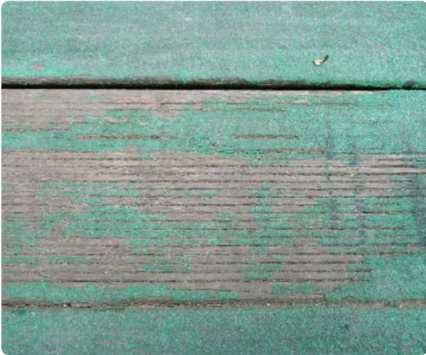
Figure 3.46: Coating degradation outdoors.
