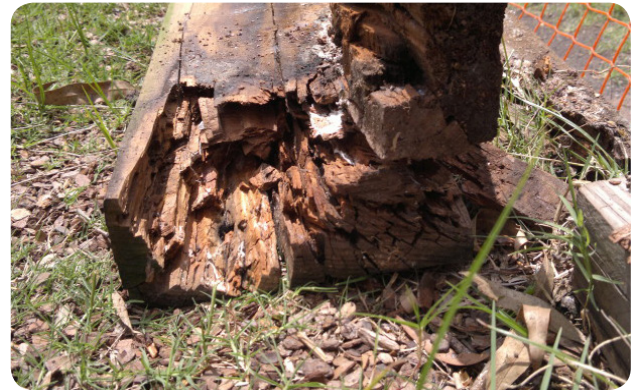
Figure 2.6: Non-compliant CCA treated pine sleepers that failed after 5 years. Sleepers contained excessive amounts of untreated heartwood.
