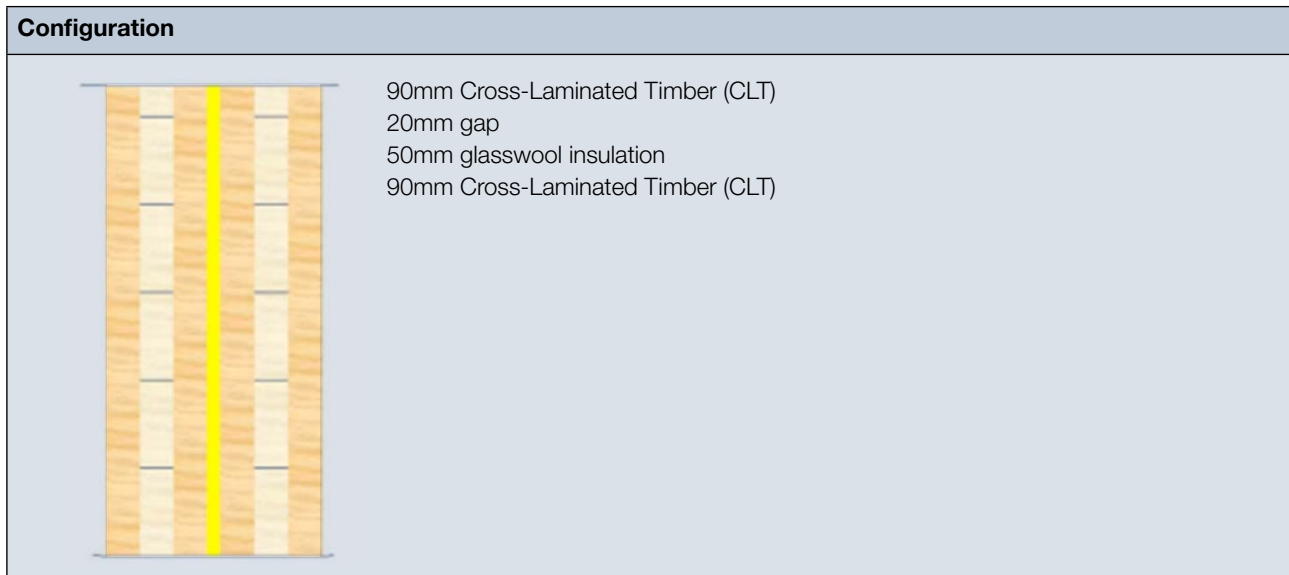
Figure 8.6: R_w \geq 50 Discontinuous Construction
