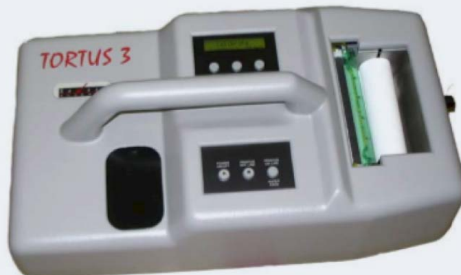
Figure 7.2: Tortus Dry Floor Friction Tester. From http://www.mastrad.com/tortus3.pdf
