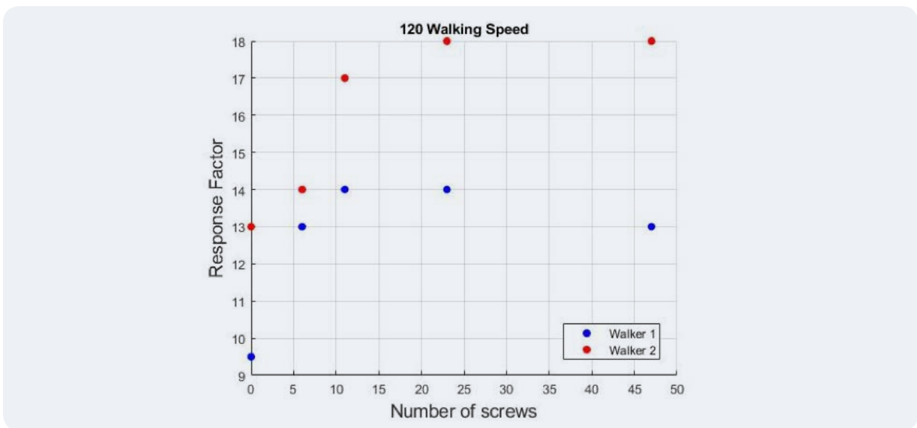
Figure 32: Response factors from walking speeds of 120 bpm on a single panel with increasing number of self-tapping screws at the support.
