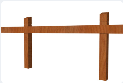
F: Recessed rails – Rebates for rails offer better support, though greater potential for decay.
