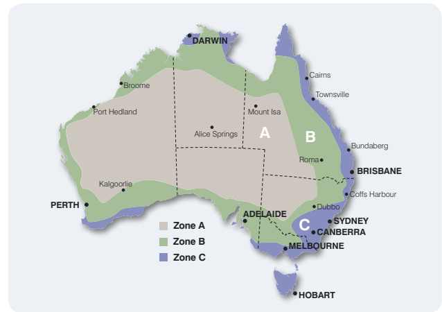
Figure 33: Hazard zone for embedded corrosion
