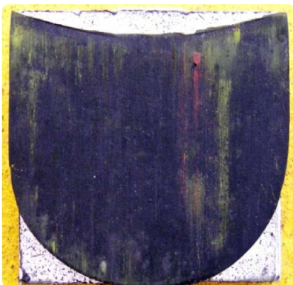
Figure 3.2: Matter between heel and pedestrian surface. Paint residue has been transferred to the test heel from the pedestrian surface.
