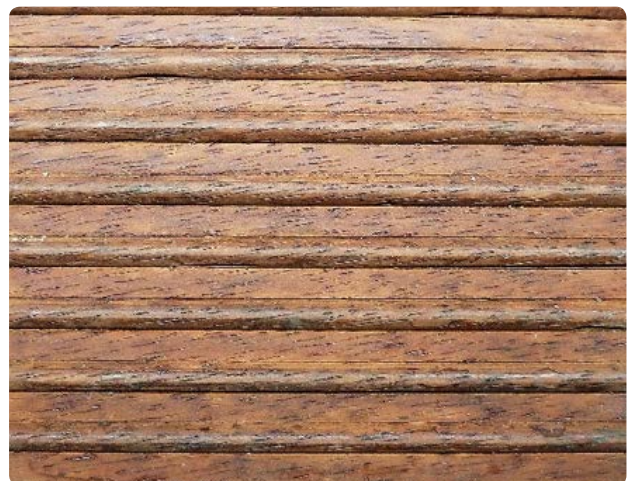
Figure 3.26: Reeded board 4 mm diameter, broadly spaced (6 mm gaps).
