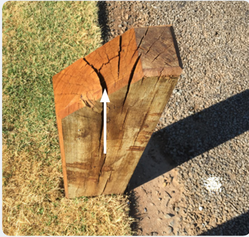
A: Radial splitting through pith
