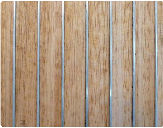
Figure 3.36: Victorian hardwood with thin metal rib inserts at 18 mm centres
