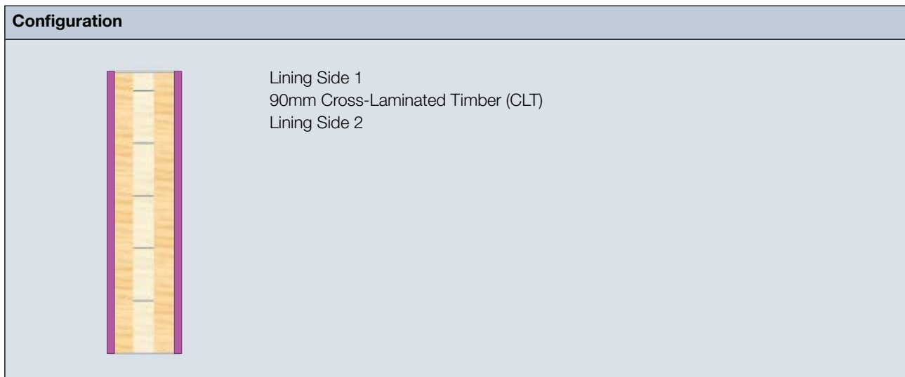
Figure 8.11: R_w + C_{tr} \geq 25
