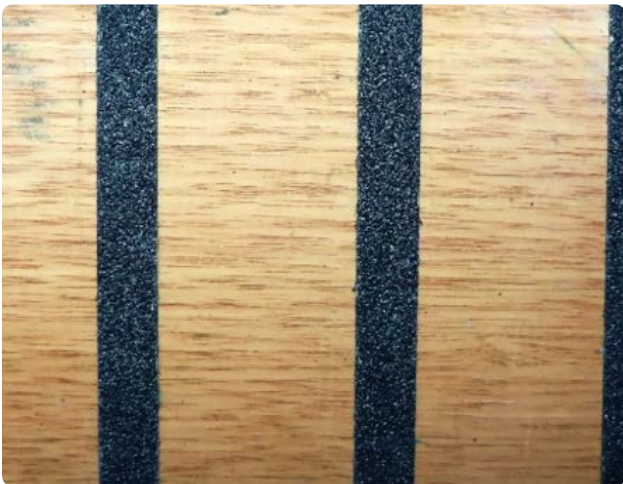
Figure 3.35: Victorian Ash hardwood with grit-tape strips.
