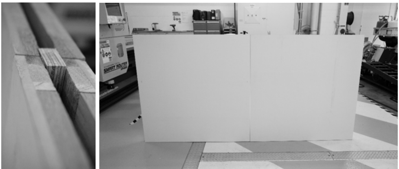
Figure 12: Partition prototype panels. Spline connector and assembly, UTS June 2016.
